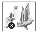
3. Remove the fibre tape.
