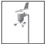
3. Slide wind vane onto the end of the plastic attachment located on the aluminium pole.
