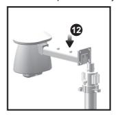
12. Slide outdoor sensor onto vertical attachment bracket.
